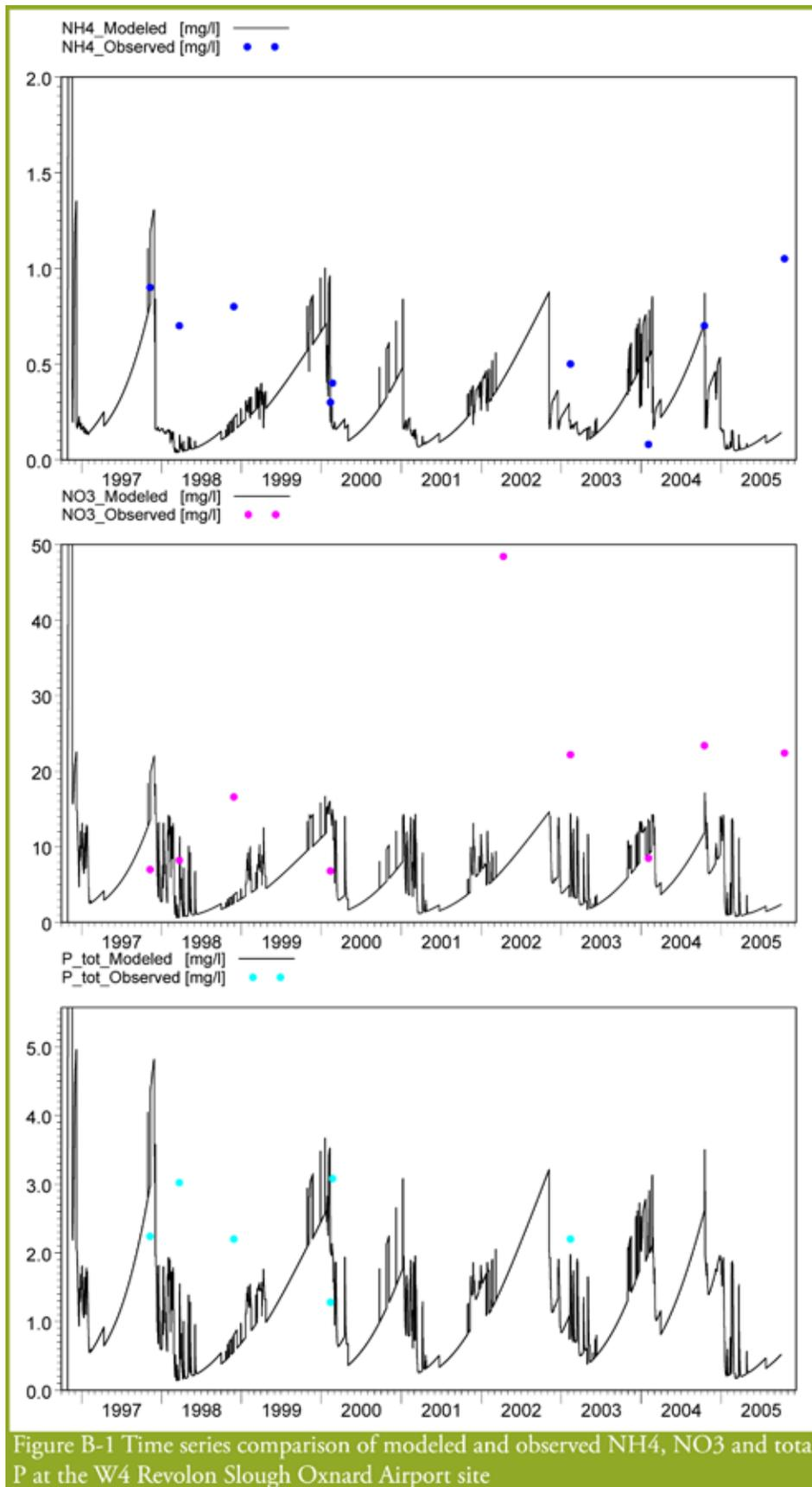
Figure B-1 Time series comparison of modeled and observed NH<sub>4</sub>, NO<sub>3</sub> and total P at the W4 Revolon Slough Oxnard Airport site
