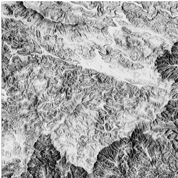
Figure 8 Unsphericity-curvature map generated from the 5 m LiDAR DEM displayed in Figure 4 . The unsphericity parameter highlights land-surface conditions that are planar in nature.
