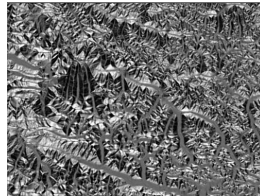
Figure 10 Second principal-component image representing anisotropic slope information extracted from local slope data over the Shimshal Valley in northern Pakistan. The slope data set was generated from a Shuttle Radar Topographic Mission (SRTM) 3 arc-second DEM. Spatial variation patterns are related to lithological units and tectonics. Less resistant metasedimentary rocks in the northeastern region and less precipitation generate a higher spatial-frequency pattern, compared with a lower spatial-frequency pattern in the southwestern region associated with more resistant lithologic units, active uplift, and greater relief.
