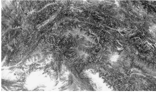
Figure 14 Sky-view factor over northern Pakistan. This parameter was computed from a Shuttle Radar Topographic Mission (SRTM) 3 arc-second DEM. Darker tones represent those areas that do not receive as much diffuse-skylight irradiance, whereas lighter tone areas receive more. The spatial patterns reveal that meso-scale relief conditions are highly variable in the Himalaya. Examination of the magnitude and spatial patterns reveals that some glaciers are receiving more diffuse-skylight irradiance than others, whereas different glaciers exhibit different trends in their sky-view-factor altitude profile. Such topographic variation regulates ablation rates and governs the sensitivity of glacier response to climate forcing. This in turn regulates melt-water production and glacial and fluvial erosion.
