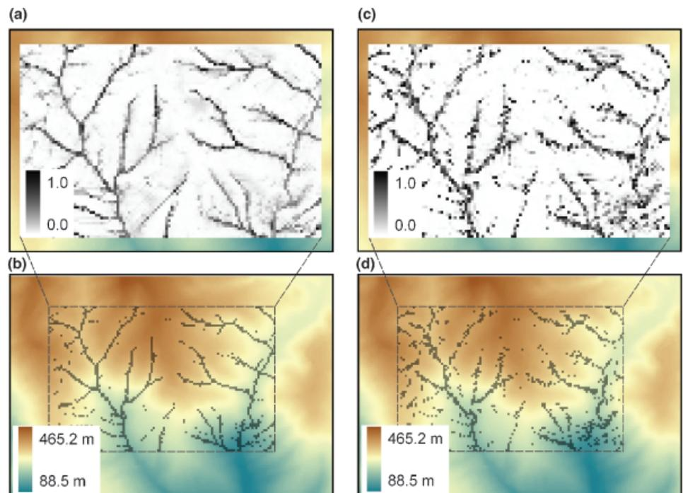
**Figure 2.** Classification results (and differences) in a small area, corresponding to Class Centers 4 and 3 in Tables 5 and 6. The maps show: (a) membership distribution of Class Center 4 in Table 5, (b) hard class map for Class 4 in Table 5 draped on 10-m DEM, (c) membership distribution of Class Center 3 in Table 6, and (d) hard class map for Class 3 in Table 6 draped on 10 m DEM.
