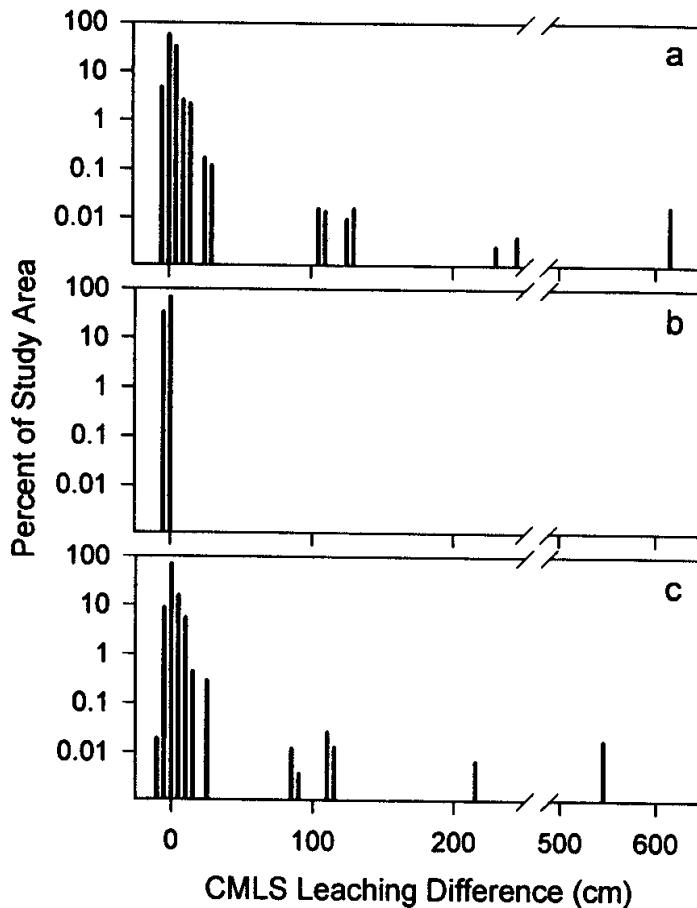
**Fig. 3. Histograms showing differences in depth of solute movement between CMLS model predictions based on MAPS/STATSGO databases and (a) MAPS/SSURGO, (b) ANUSPLIN/STATSGO, and (c) ANUSPLIN/SSURGO databases.**
