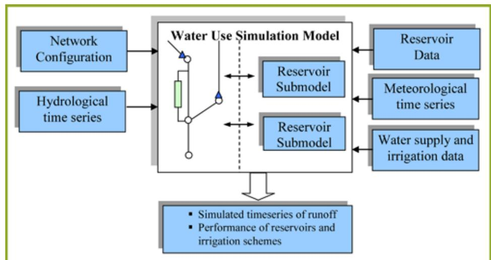
Figure 1 MIKE BASIN's water allocation modeling structure (DHI 2007)
