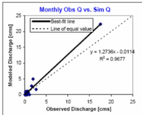
Figure A-2 Calibration results for USGS 11108000/F92-R Santa Clara River near Saugus CA gauging station
