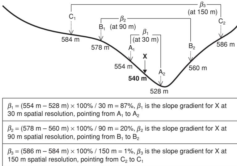
**Fig. 23.3** Scale effects of terrain analysis. Slope gradients ( $\beta_1$ ,  $\beta_2$ , and  $\beta_3$ ) for the same point B (or  $d$ ) are defined in different ways due to the change of spatial resolution. The resultant slope gradients are different not only in magnitudes, but also in terms of topographic meanings
