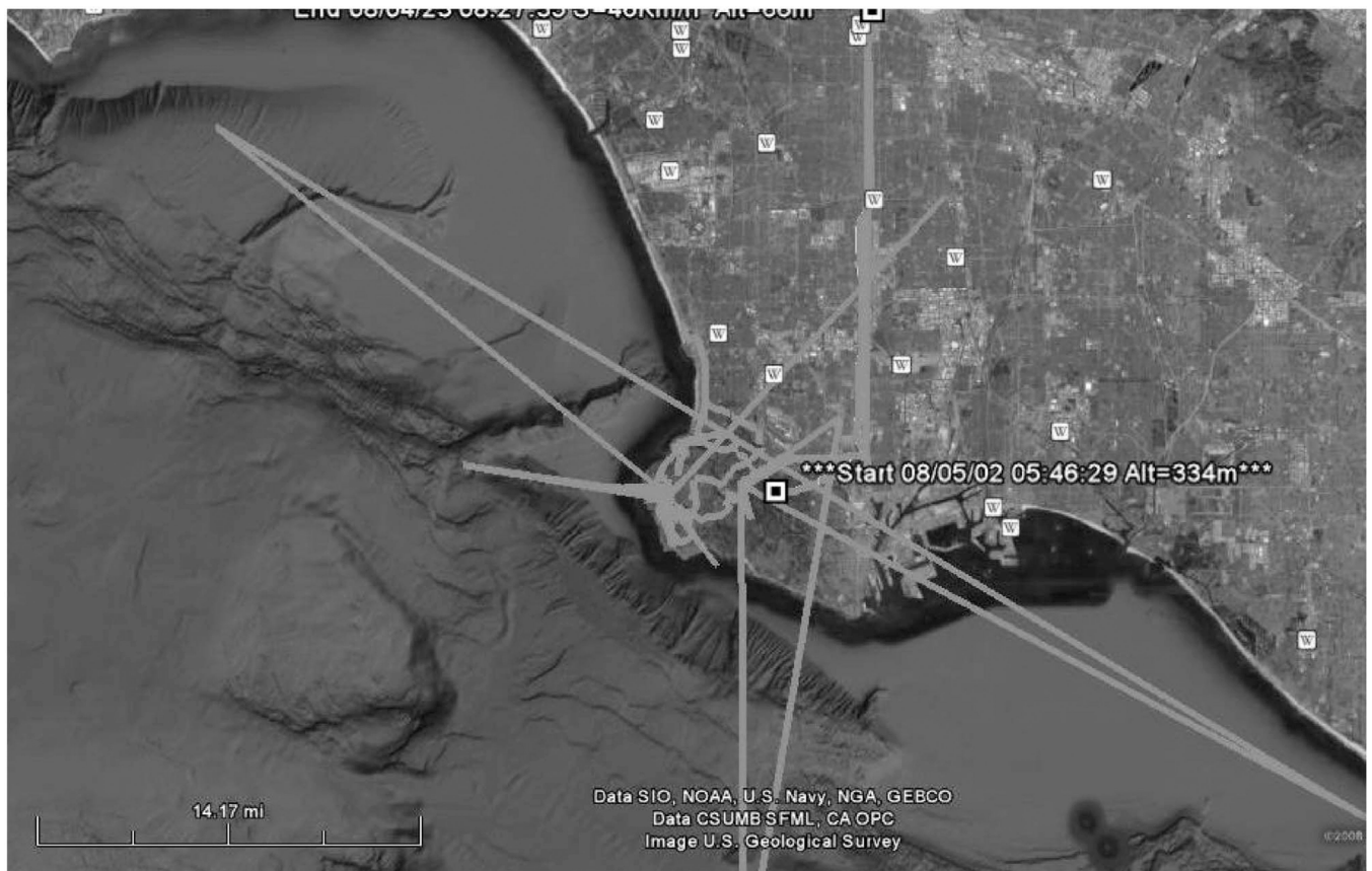
Figure 2. Representation of global positioning system (GPS) raw data, showing example of data with travel between locations on land and well into the ocean between 15-s recordings.
